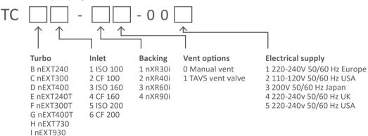
nEXT730/930 variants cannot be used with 110-120V 50/60 Hz USA voltage Important note: System is not UL certified.
