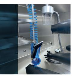
Moreover, a gas gun serves as a valuable tool for efficiently removing particles from surfaces, including substrates, by blowing them away.
