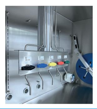
Our complete solvent purification systems, designed to eliminate oxygen and moisture from solvents, can be seamlessly integrated with an MBRAUN glovebox or utilized as an efficient standalone unit.
