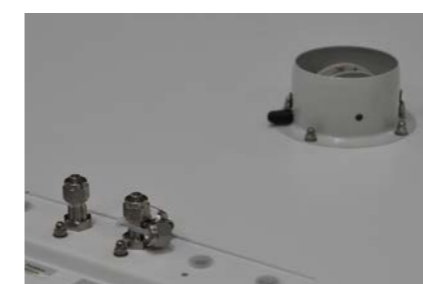
Exhaust on the top, and optional connectors for integration to a glovebox
